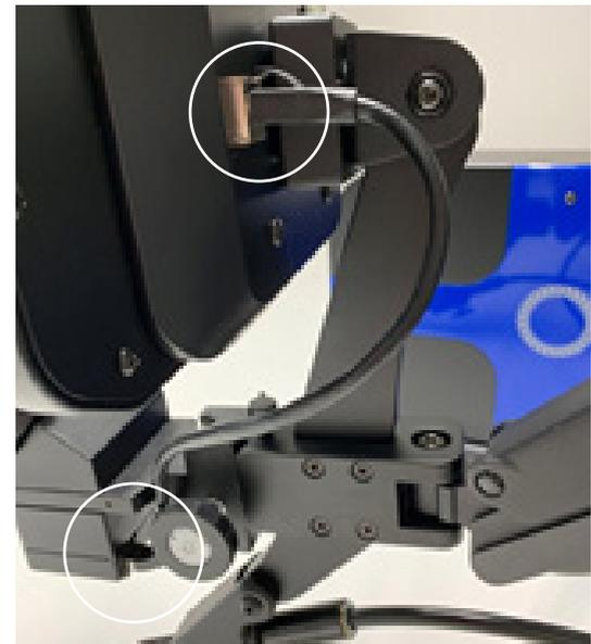
*Figure 7.3 After installing the rubber eyepiece covers, use the Shutter Cable to connect the Touchscreen to the bottom of the microscope head.*
