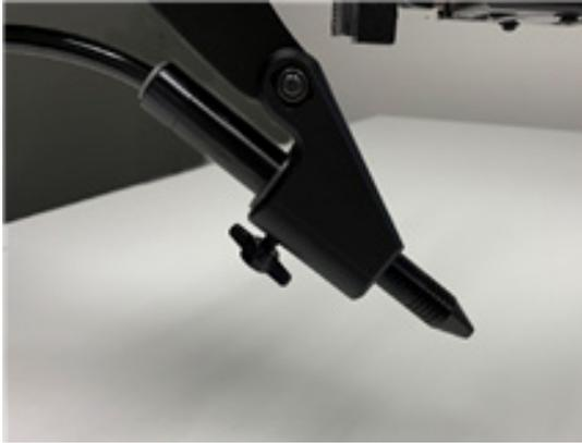
Figure 8.1. Mount the Welding Stylus to the holder below the microscope.
