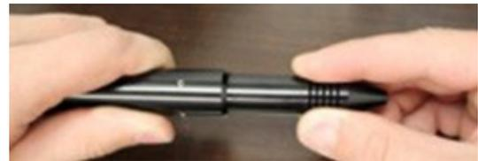
Figure 9.2. To install the electrode, first remove the stylus shaft from the stylus hull by pulling them apart.
