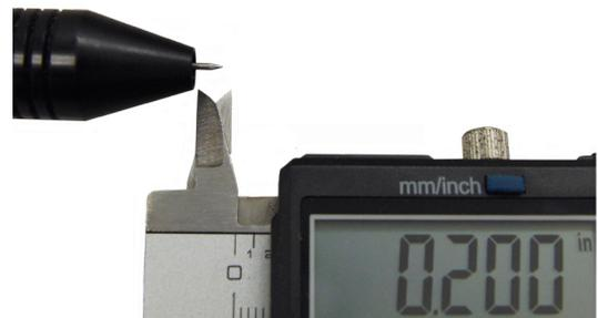
Figure 9.4. The electrode should protrude past the stylus hull 1/8 to 1/4 inch (3.175 to 6.35mm).
