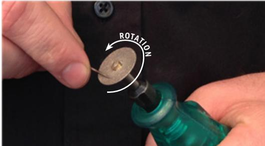
Figure 12.1. A sharp electrode tip improves arc initiation and results in a better overall weld.
