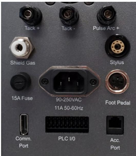
Figure 10.3. Power Supply back panel.
