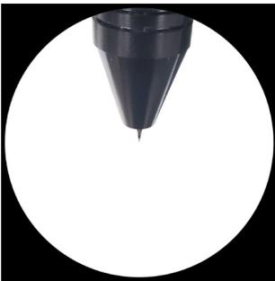
Figure 8.3. When looking through the microscope, the stylus should appear in the center of your focus, as shown here.
