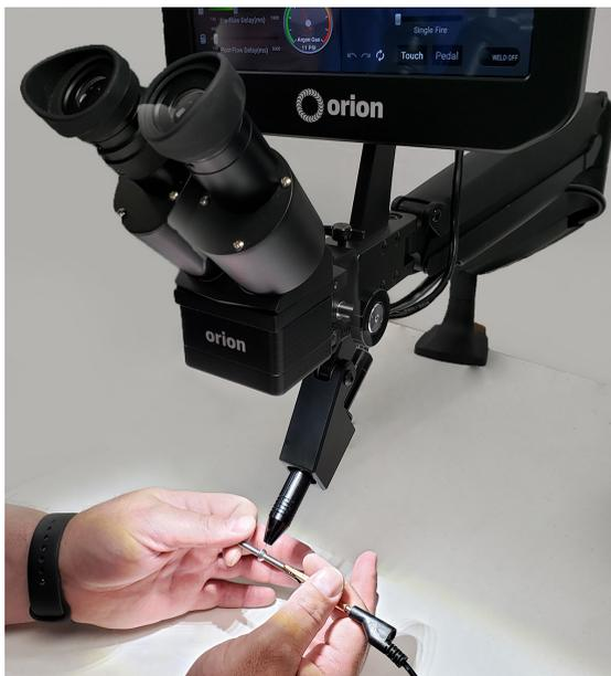
Figure 14.1. Rest your hands on the table and position the workpiece close to, but not touching the electrode, then look through the microscope.
