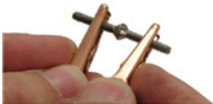
Figure 42.2. In Tack mode, simply touch the two workpieces together to initiate the weld, as shown in the example above.
