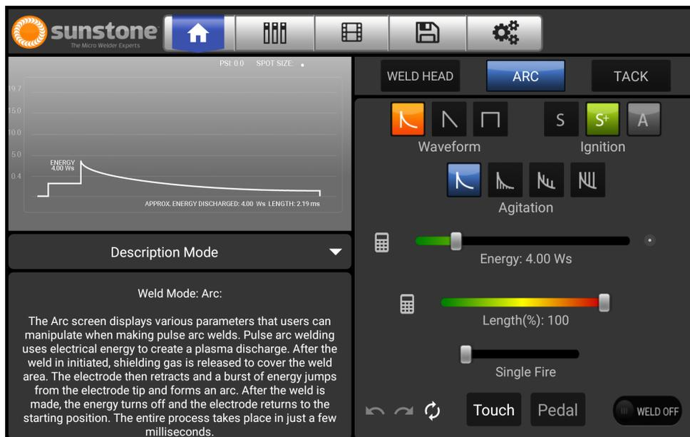
Figure 20.1. When you touch "ARC", the button will turn blue and new parameter controls will appear for Waveform, Ignition, Agitation, Energy, Length, and Weld Speed.
