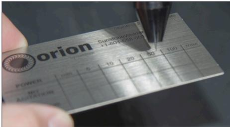
Use the provided stainless steel weld plate (as shown above) as a guide to try different settings and practice weld placement. Make several welds on the weld plate to get comfortable with the stylus and the effects of different weld parameters.
