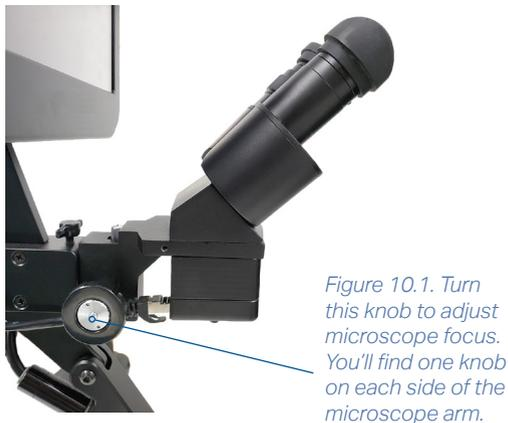
Figure 10.1. Turn this knob to adjust microscope focus. You'll find one knob on each side of the microscope arm.
