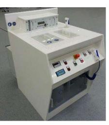
$\mu$ Galv R&D is a turn-key electroplating system for various metals (Au, Ni, Cu) as well as additional rinsing cells or quick dump rinsers are available.
